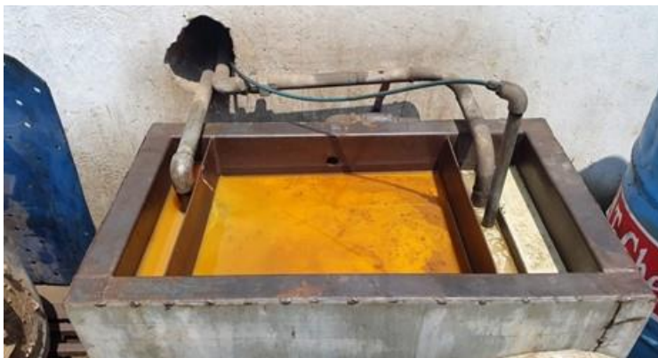
Oil Filtration system for degreasing bath
