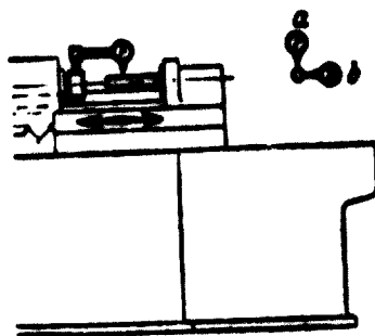
Fig. 72. Parallelism between the Spindle Axis and the Direction of the Table Traverse
