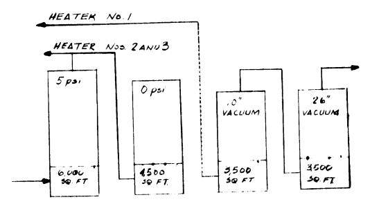
Total evaporation obtained equals 83, 289 pounds per hour with an evaporation rate of  $\frac{83, 289}{17, 500}$  or 4.75 pounds per hour per square foot.
