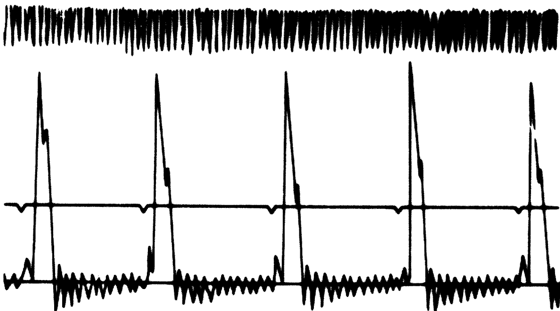
Figure 4. Oscillogram of thread tension in the lock-stitch sewing machine
