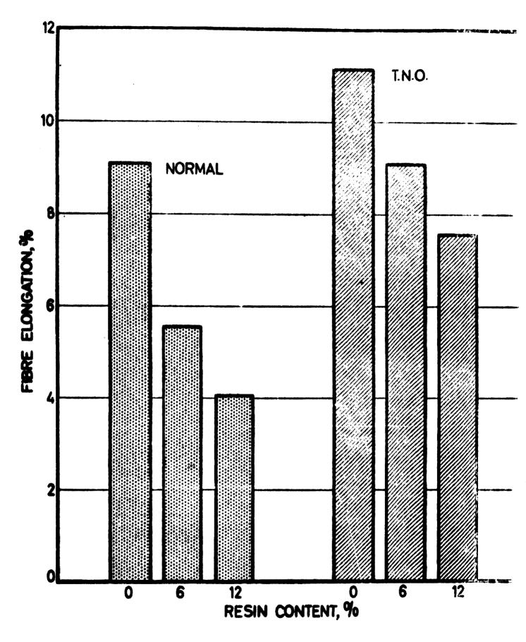
Fig. 2 Dependence of ootton fibre elongetion at break on regin content
