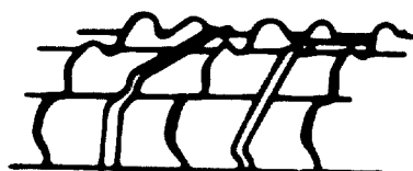
Figure 2. Formation of sheds by warp discs
