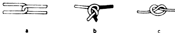
Figure 1. Loop (a), knot (b) and tie (c) forms of specimens tested for strength
