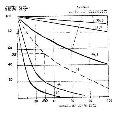
The dotted line indicates, that a circuit, consisting of 30 components, each with an average reliability of 98%, is likely to have a total reliability of orly 55%, which is far from acceptable in most industrial applications.
