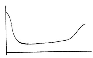
The vertical axis gives the number of failures per time unit, the horizontal axis is the time of operation.
