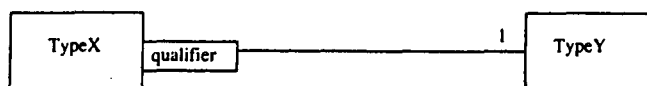
(b) One object of TypeY is linked to one object of TypeX via an identifier
