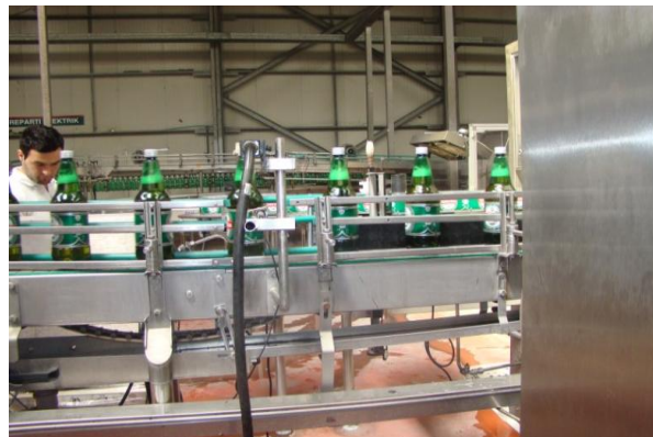
After flow control valves: Equal filling at PET line
