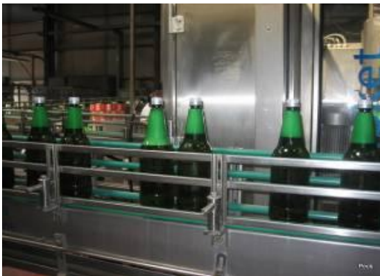
Before flow control valves: Uneven filling at PET line
