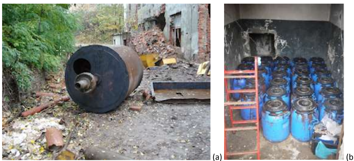
Figure 1: (a) TNT chipping equipment cleaned by hand, steam and flame (to remove trace elements of TNT), and (b) TNT securely stored in temporary storage
