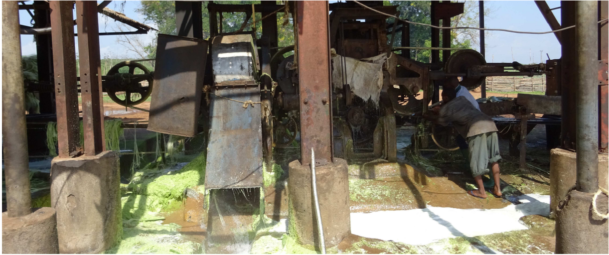
Figure 9: Decorticator/Corona at Maboga in Mazinde Estate
