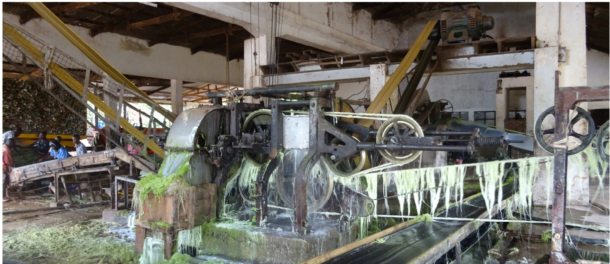
Figure 2: Sisal decortication unit at Hussani
