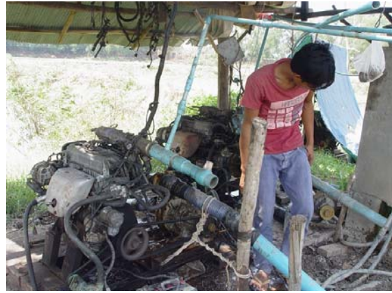
Figure 76: Biogas fuelled water pumps
