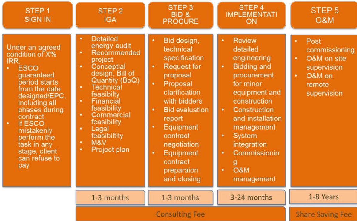
Figure 3.4: Stages of implementation of energy efficiency projects using ESCO services
