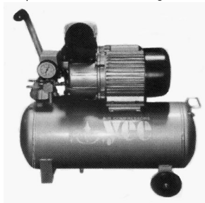
Figure 28 Reciprocating air compressor
