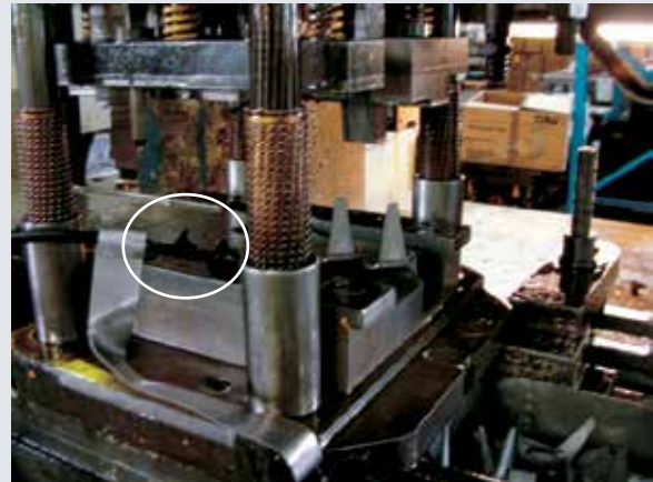
The inappropriate use of compressed air as it was used to blow parts out of the press. This cost the company an estimated R5000.00 annually
