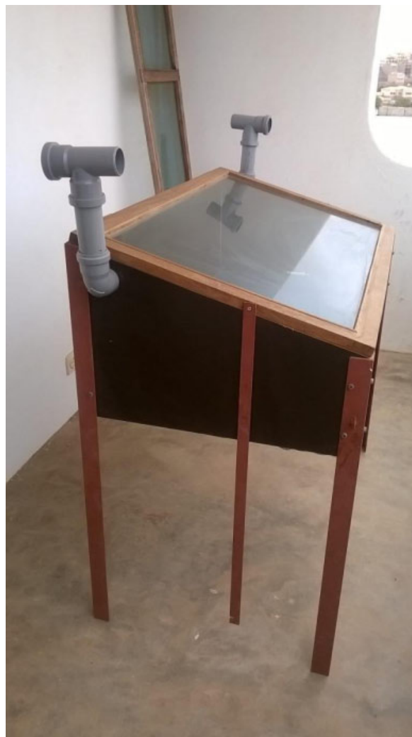
Figure 21: Solar dryer for home use (fruit drying) – photo provided by owner of dryer (Ms. M.M. Estrela)
