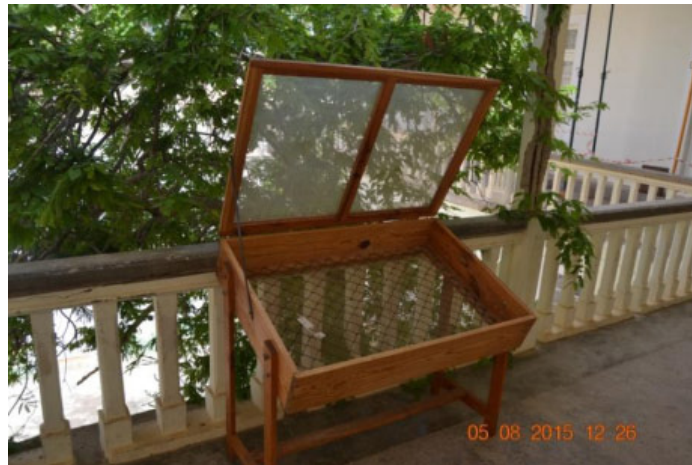
Figure 20: Fruit dehydrator used by a NGO in S. Vicente to dry fruits (experimental) – photo taken at Mindelo International School of Arts
