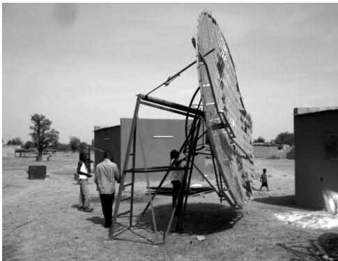
PICTURE 1. SOLAR THERMAL PARABOLA FOR SHEA NUT PROCESSING. MADE BY ISOMET IN DABARÉ, BURKINA FASO. PHOTO BY GREGORY MILLER, SNV.
