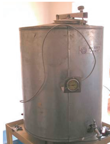
Fig. 5.10 Insulated filling tank
