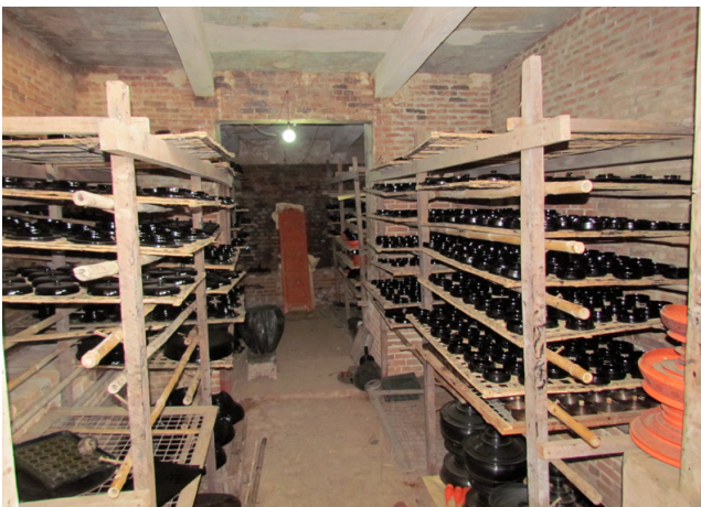
An underground drying cellar, which is one of the most important steps in the lacquerware production process
