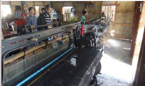
P 23: Semi Automatic Loom
