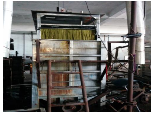
P14: Two Colour Hank Yarn Dyeing Machine
