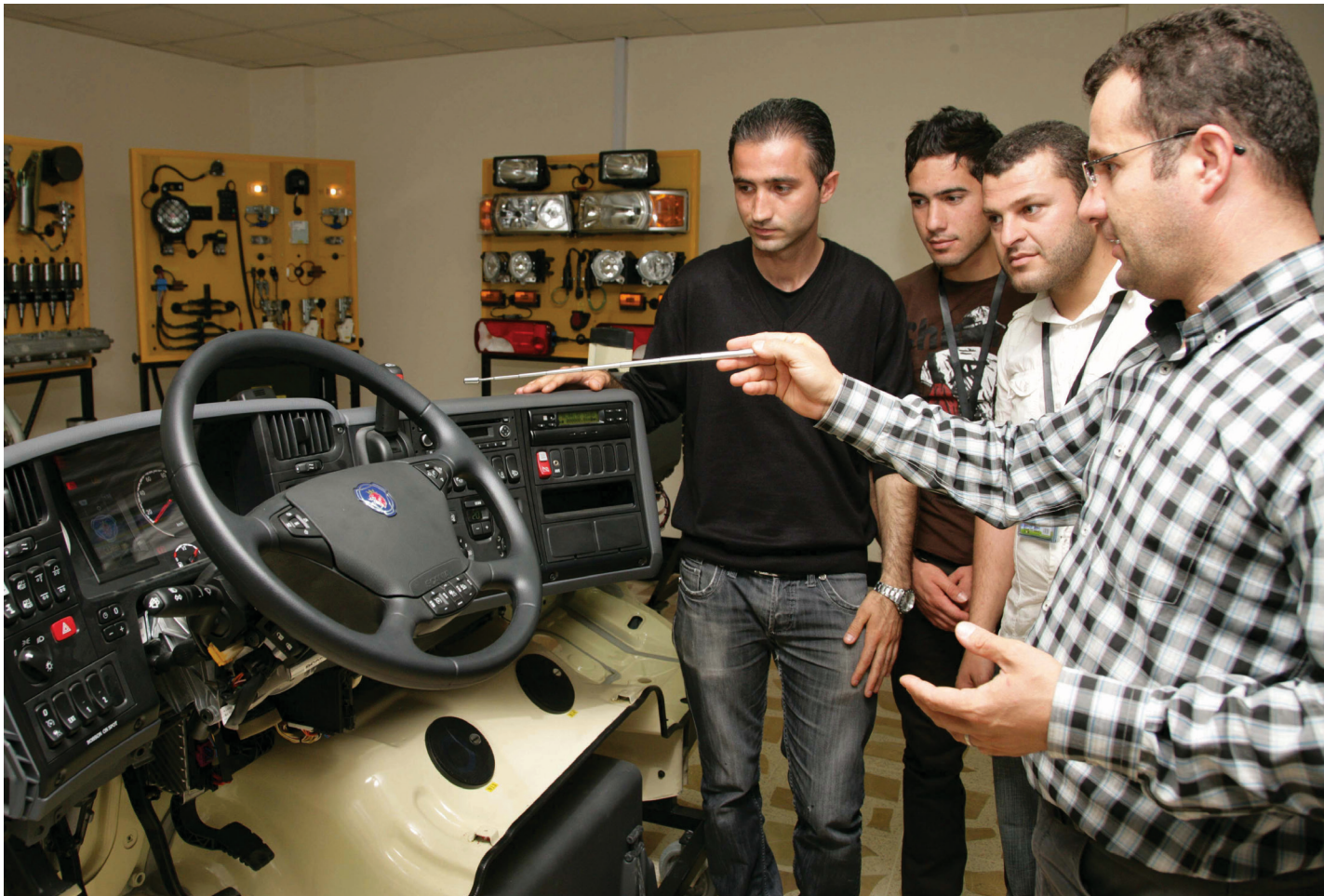
Photo 2: Zana Mustafa Rafiq, teacher at the Swedish Academy for Training in Iraq, instructing students on the layout and operations of a Scania truck dashboard
