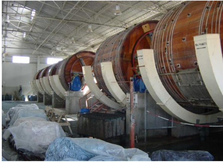
Figure 25. A battery of drums with semi-circular float collection gutters
