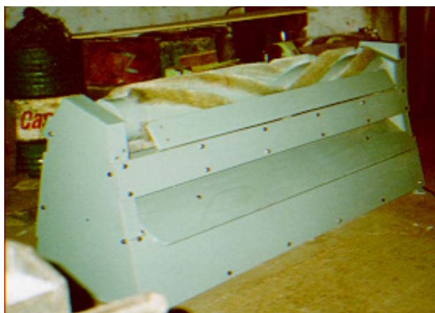
Figure 20. Brush type desalting machine
