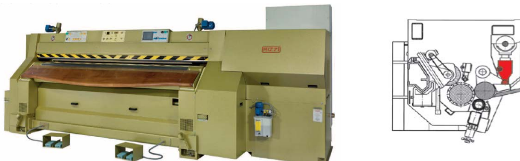
Figure 37. Shaving machine with cross-section schematic view
