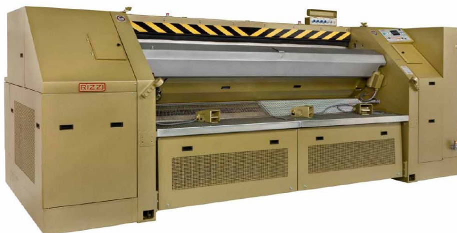
Figure 17. Through feed fleshing machine
