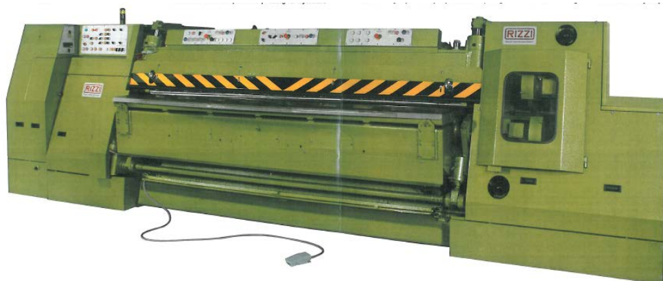
Figure 31. A splitting machine for both ex-lime and wet blue splitting
