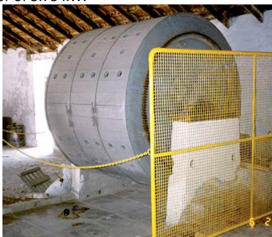
Figure 19. Old wooden drum converted into a desalting drum
