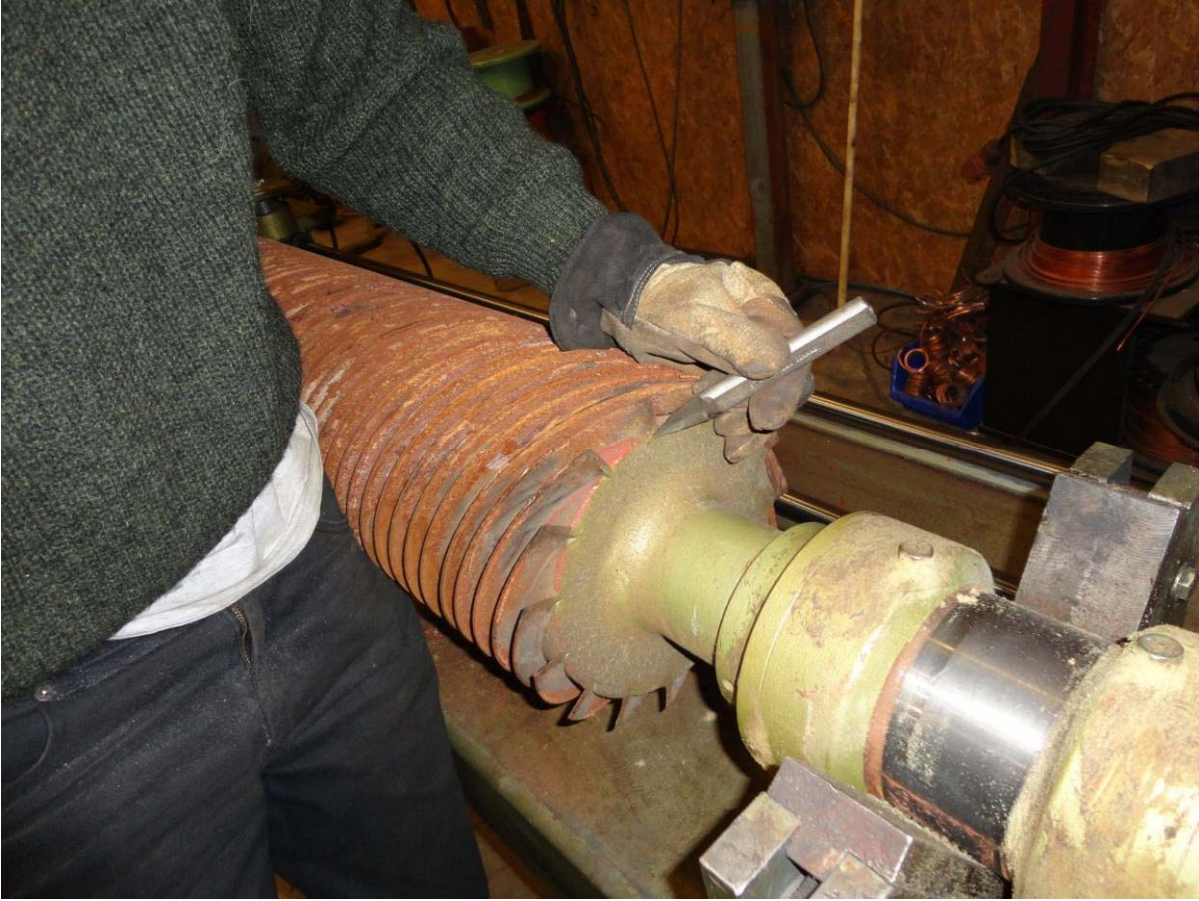
Figure 6 How to start removing the caulking by using chisel
