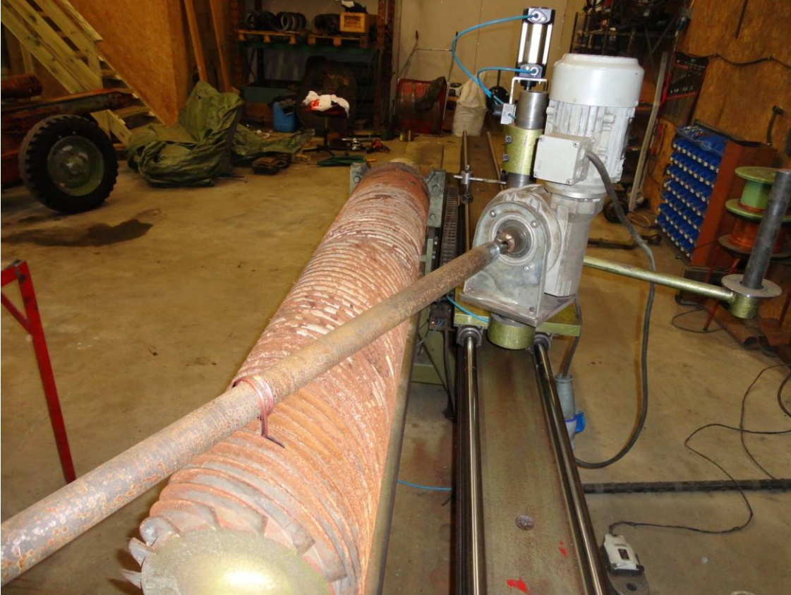
Figure 29 Rolling caulking on pipe
