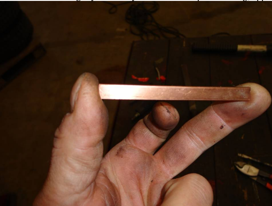
Figure 22 Strip of caulking for initial fastening of blade
