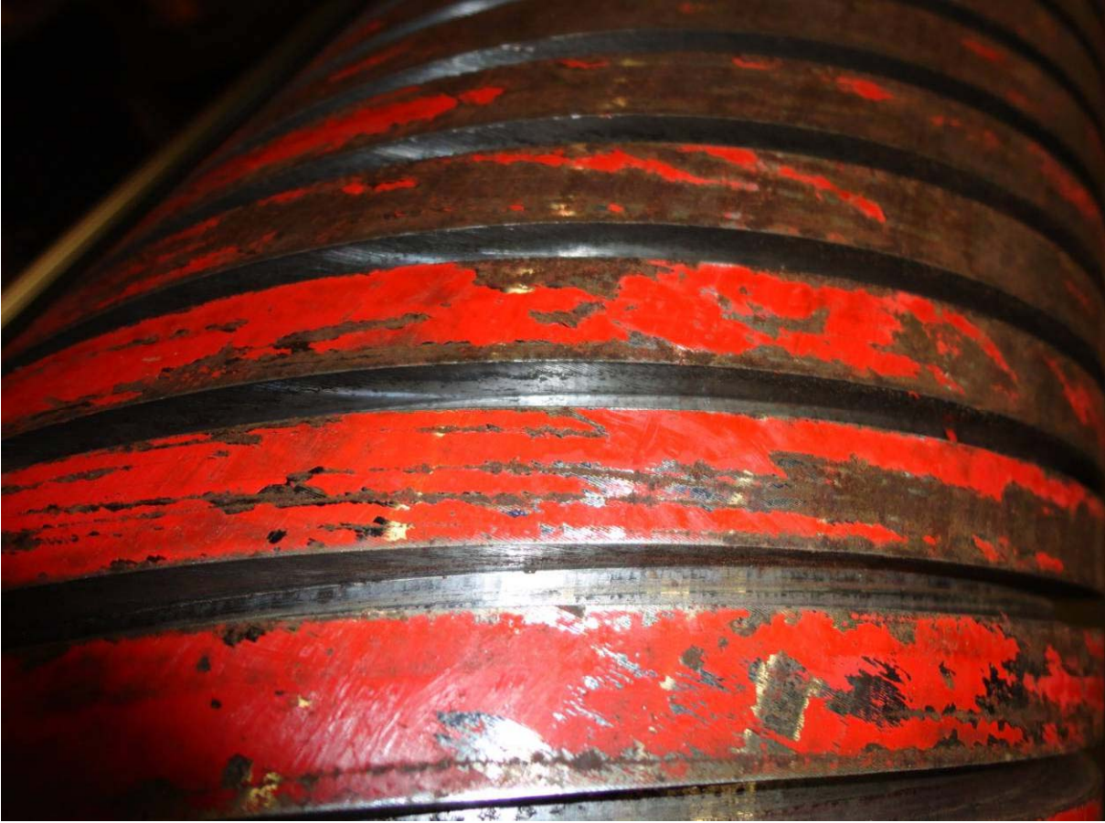
Figure 17 Undamaged grooves after removal of blade and caulking
