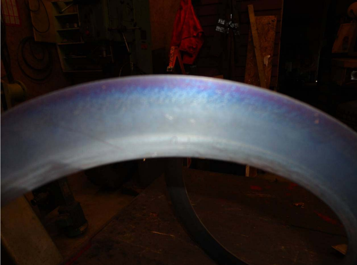
Figure 19 Blade displaying colour patterns from hardening and tempering.
