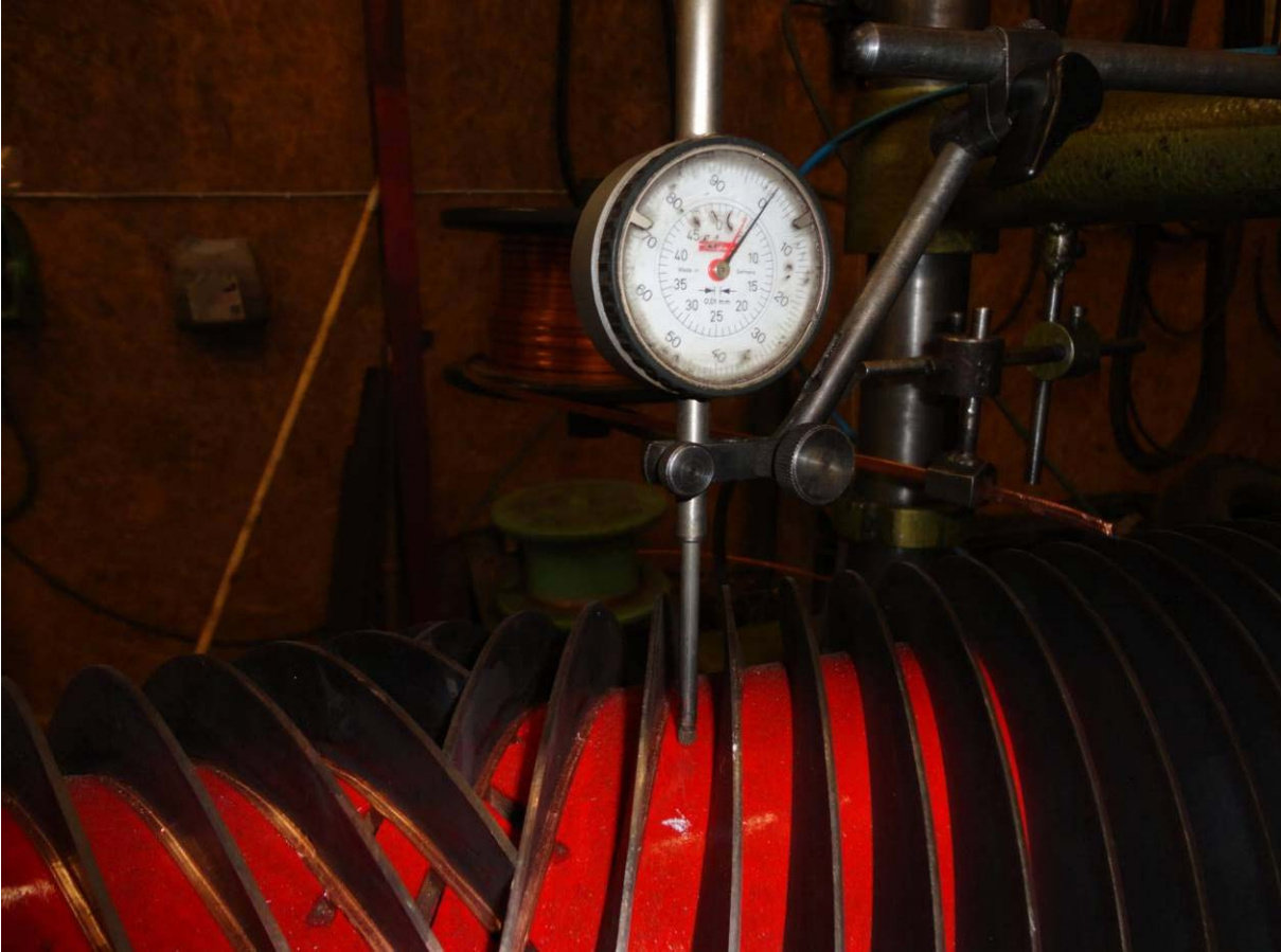
Figure 47 Use a micrometer on cylinder surface. Measure between all the blades to check the "true" circle
