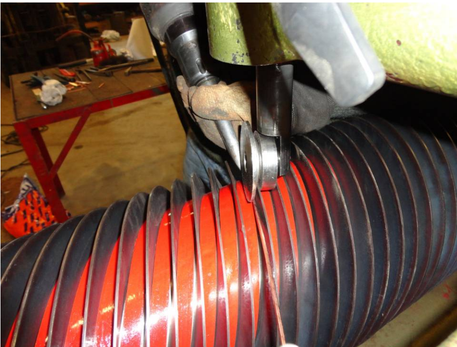
Figure 42 Continues hammering on caulking, while cylinder rotates. Fresh caulking fed automatically
