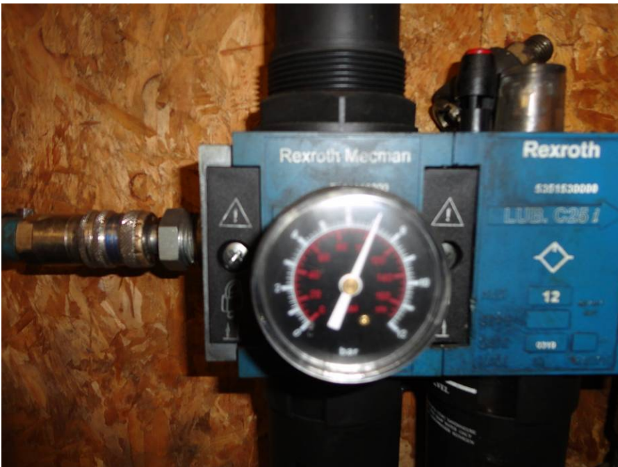
Figure 39 Pneumatic pressure on hammer, 7 bar
