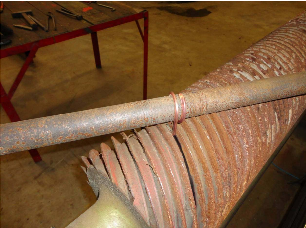
Figure 12 Caulking being rolled on pipe
