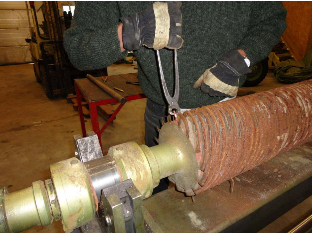
Figure 9 Use of pliers minimizes the risk of breaking the caulking
