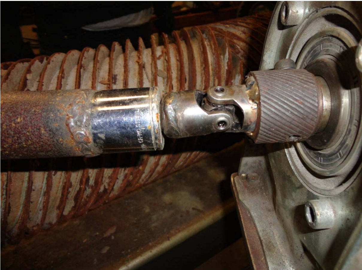
Figure 11 Connect the pull off pipe to the pulling device/motor
