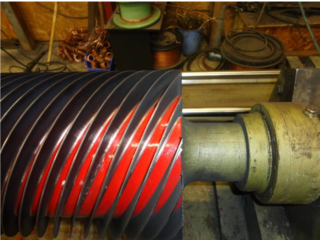
Figure 46 cylinder after cutting the blades
