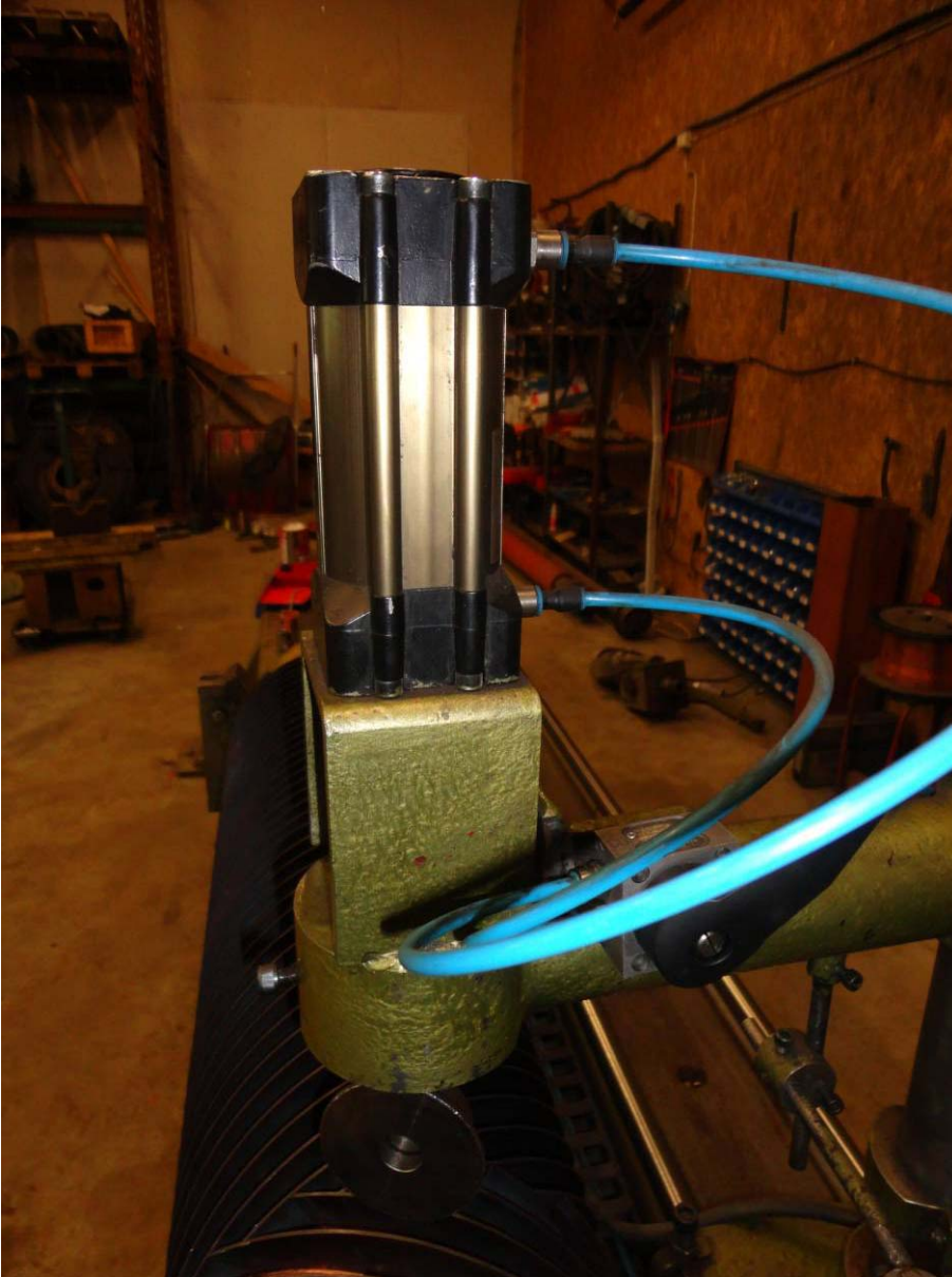
Figure 40 Pneumatic cylinder and wheel for blade clamping
