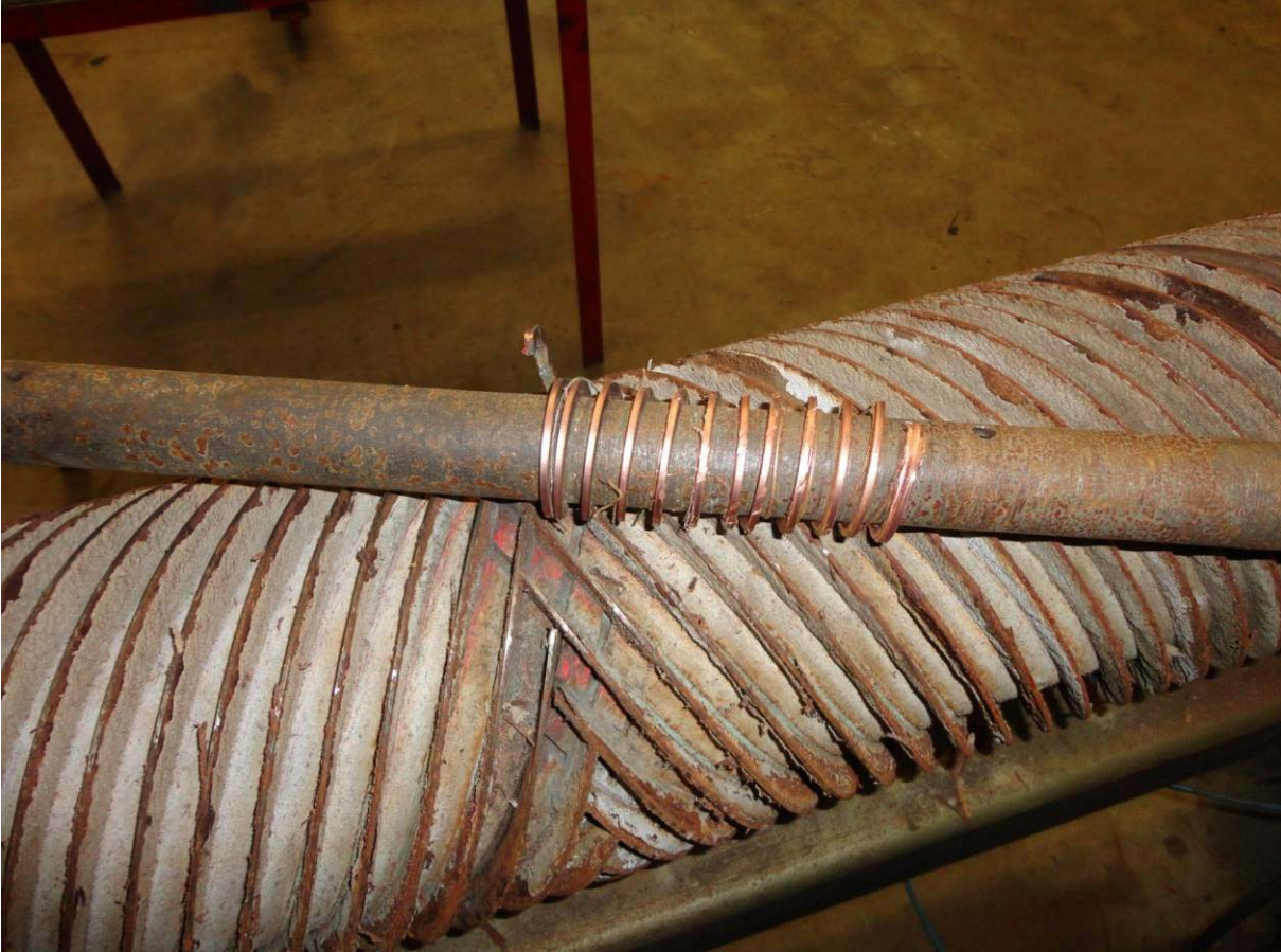
Figure 13 The caulking has been removed from one blade.
