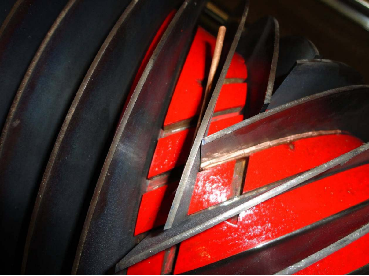
Figure 21 A good fit in centre of cylinder is achieved by proper end adjustment.
