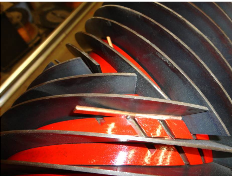
Figure 37 Two first blades are aligned and fixed
