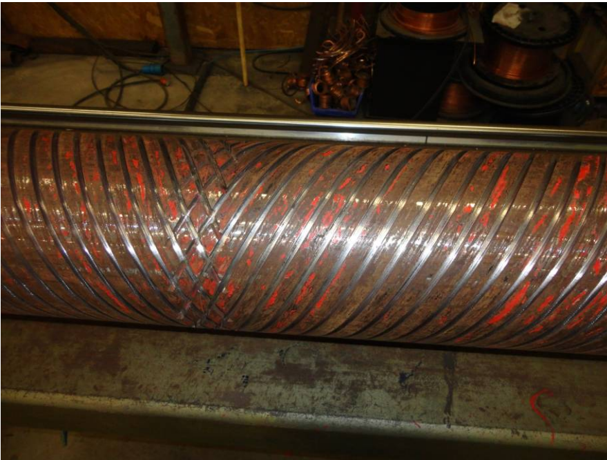
Figure 31 Cylinder with blades removed and cleaned
