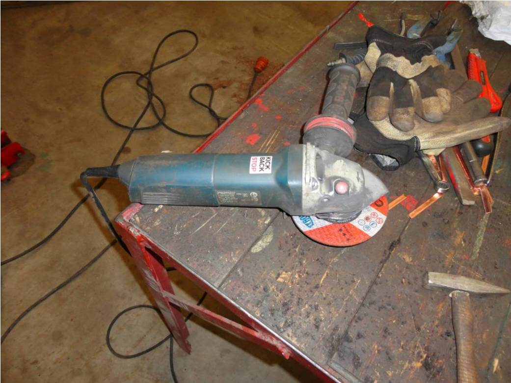
Figure 45 Disk grinder to be used for cutting excess blade length
