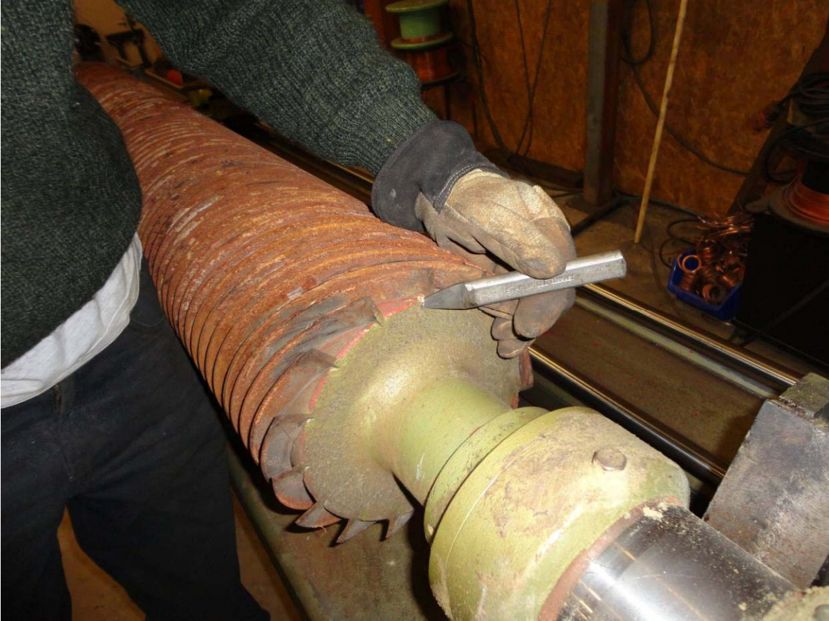
Figure 7 Be careful to loosen chisel on regular intervals to avoid damage to cylinder
