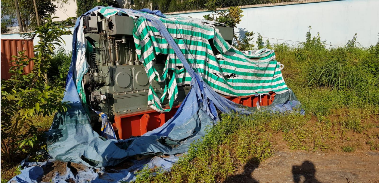
Condition of storage of 1 MW engine
