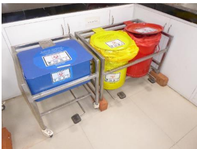
The wheels have broken off the bin set on the right
