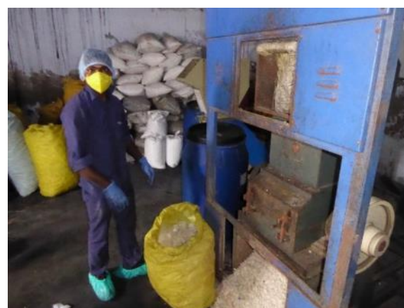
Shredding plastic for recycling
