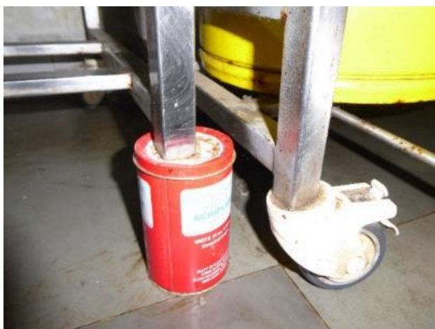
Project provided bins often lose their wheels. Note that the wheels are difficult to keep clean.
