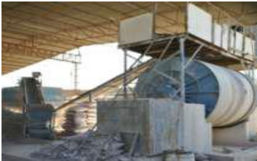
Image 2: Slurry mixer at ceramics factory in Morbi Cluster
