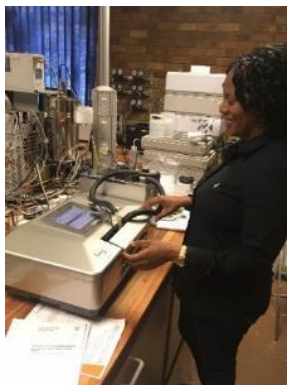
Optical rotation equipment testing essential oils, NMISA Organic Analysis Laboratory, 19.9.2023, Photo by evaluator
