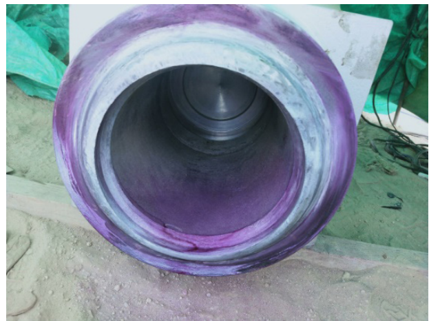
PT inspection of chrome-molybdenum steel P91 groove
