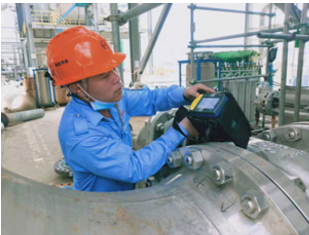
PMI, PT inspection of components and welds after pipeline installation
