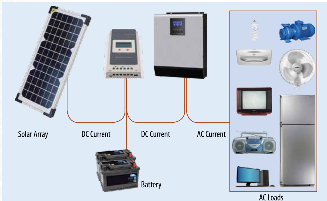
Figure 36: Show The general framework of any system using solar cells as an energy source.
